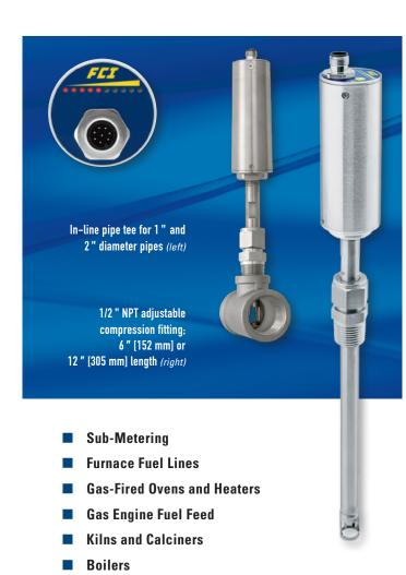
The FS10i is a compact, economical solution to natural gas flow metering. Utilizing application proven thermal dispersion technology, the FS10i provides a highly accurate and repeatable linearized 4-20 mA output of flow rate. Additionally, for applications benefiting from a high or low flow alarm point, the FS10i includes a user programmable 1A SPDT relay output.
