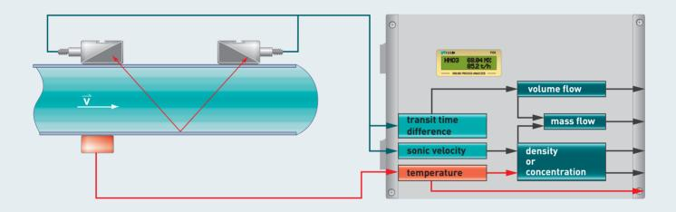
Two ultrasonic transducers are mounted to the pipe wall, and are alternatingly sending and receiving ultrasonic signals. Measuring the difference in the transit time between the two signals, the flow velocity (v) and the volume flow, based on the pipes inner diameter, are accurately calculated.
