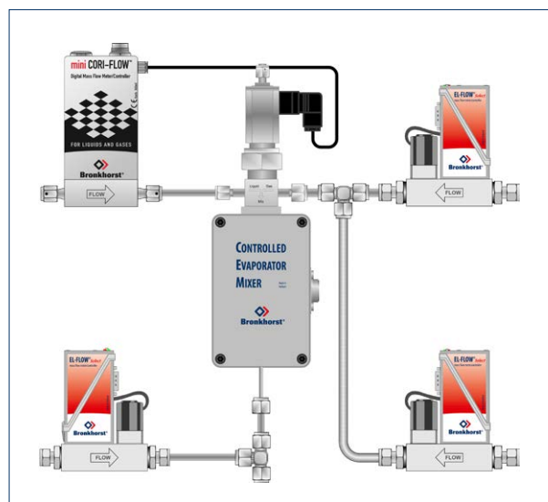
Dual carrier gas supply with dilution, Coriolis liquid flow meter
