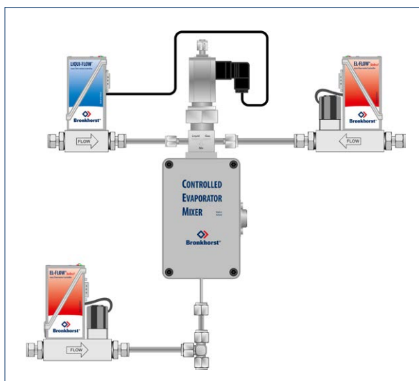
Single carrier gas supply with dilution, thermal liquid flow meter
